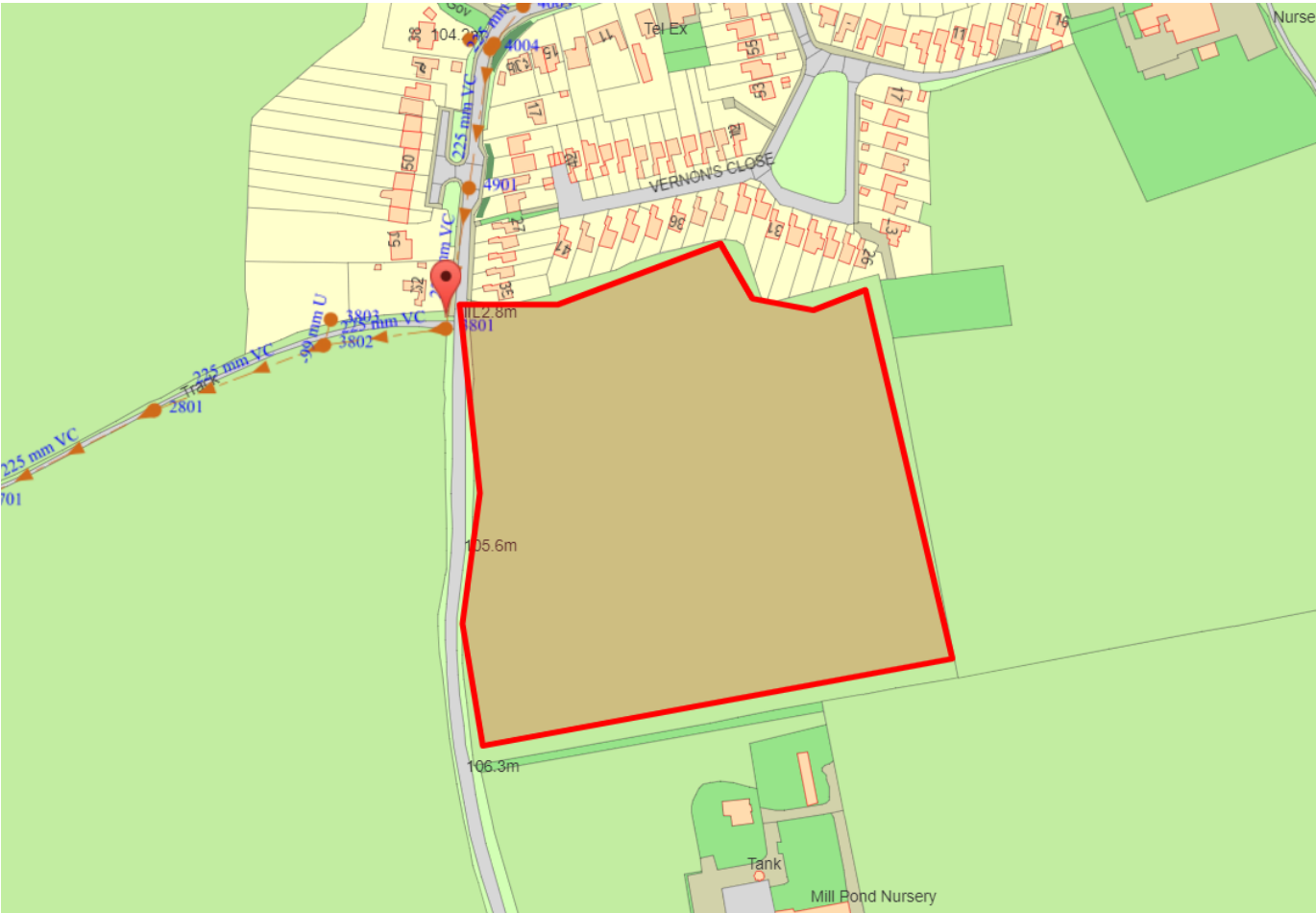
Figure 1: Showing your water recycling foul point of connection
