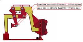
If the adjustment is required to be undertaken on-site ensure this is carried out whilst the lifter is stabilised and contained within its stillage. Two operatives are required to perform the task. Remove securing bolt and collar and carefully take out 40mm diameter pin. Re-position the clamp to the required hole and slide the pin back in place, slip over the collar and tighten M10 bolt.
