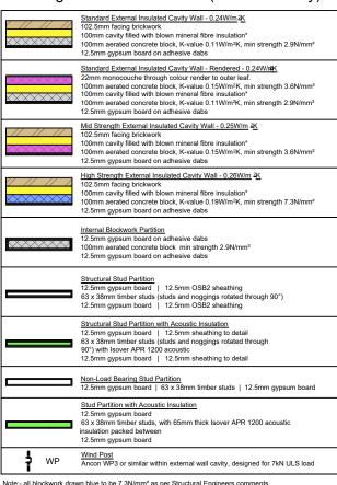
Note:- all blockwork drawn blue to be 7.3N/mm² as per Structural Engineers comments. Refer to relevant Construction Specification for either and 2021 Build regs for further details
