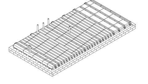
Closure Blocks are only included for around the perimeter, as is highlighted on our design. If you would like additional Closure Blocks for internal walls, please contact Litecast.
