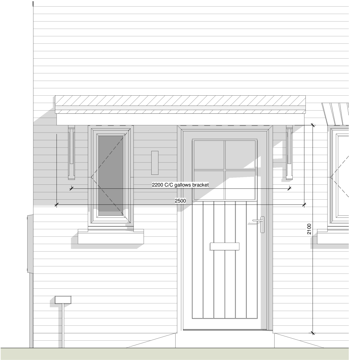
1 Canopy - Front Elevation 1 : 20
