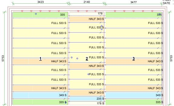
DESIGN ALLOWS FOR AN ADDITIONAL 1.0KN/m<sup>2</sup> LOAD FOR NON-LOADBEARING STUDWORK PARTITIONS IN BAYS 1, 2, 3
