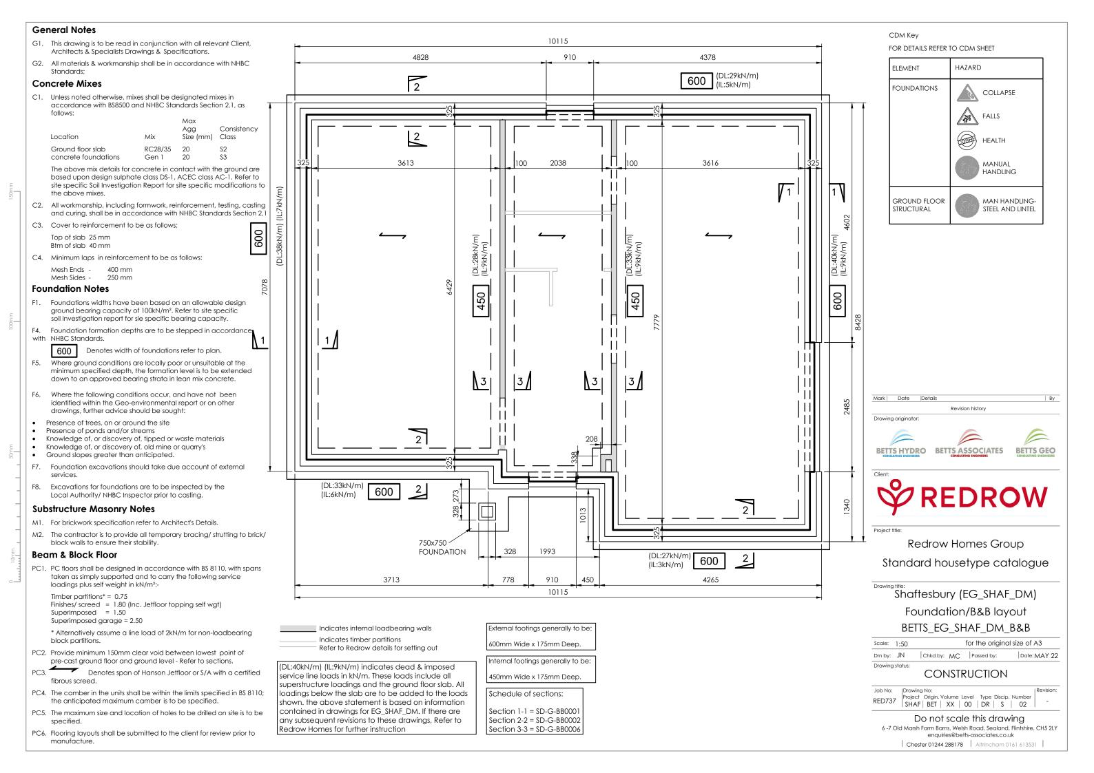
Movement joints and bed joint reinforcement indicated apply only when house is built as shown, if house is built as a semi-detached or terrace refer to block drawings for details.
